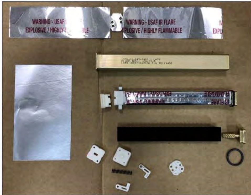
Figure 7-18. MJU-73/B with Components Spread Out
