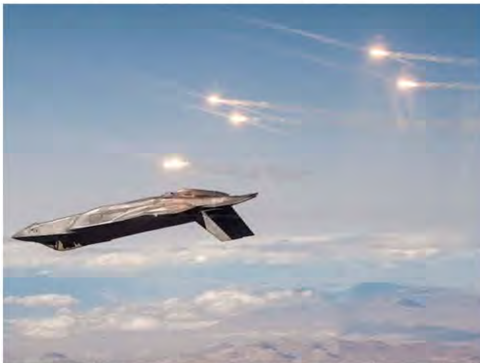
Figure 7-1. Aircraft Deploying Flare Countermeasures and Maneuvering to Avoid a Simulated IR Missile Threat During Training
