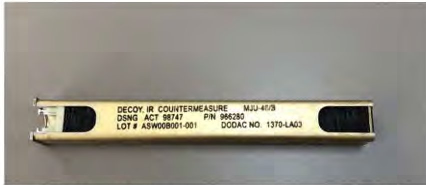
Figure 7-25. MJU-46/B Spectral Decoy
