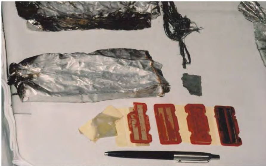
Figure 8-3. MJU-7 End Caps (Red) and Wrapping Material
