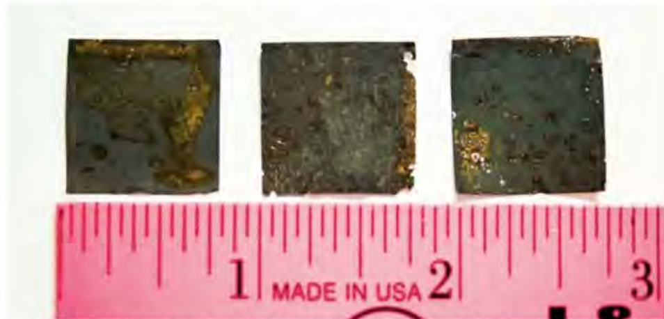
Figure 7-24. Pyrophoric Iron Foils After Spectral Decoy Deployment and Some Weathering
