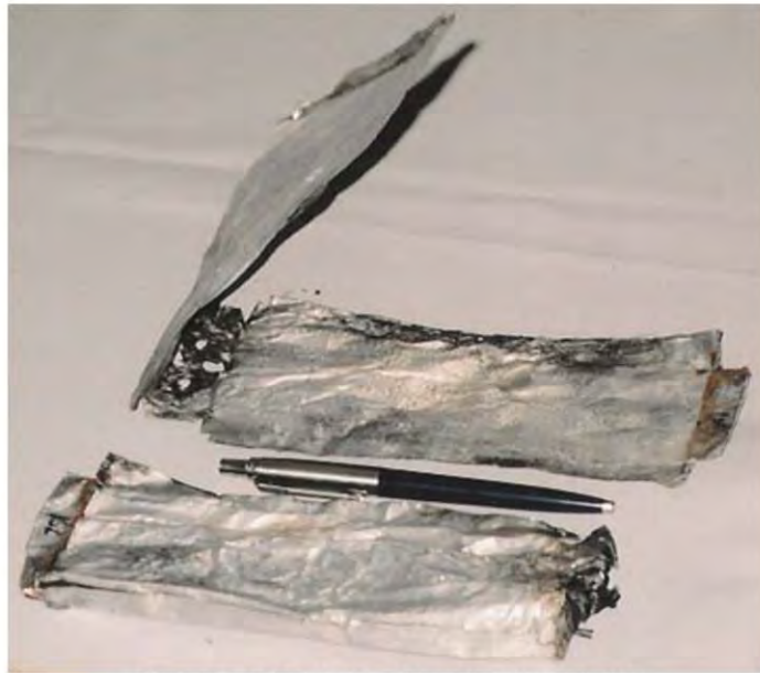
Figure 8-2. MJU-7 Residual Flare Wrapping Materials
