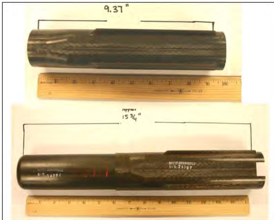
Figure 7-20. MJU-39A/B and MJU-40A/B Flares
